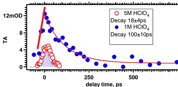
Figure 2. The decay kinetics of observed in pulse radiolysis of 1 and 5 mol dm<sup>-3</sup> solutions of perchloric acid in water (filled squares and empty circles, respectively). The electron rapidly decays in a reaction with hydronium ion.
