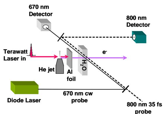
Figure 1. Experimental Set-up for ultrafast pulse radiolysis using a laser wakefield accelerator.
